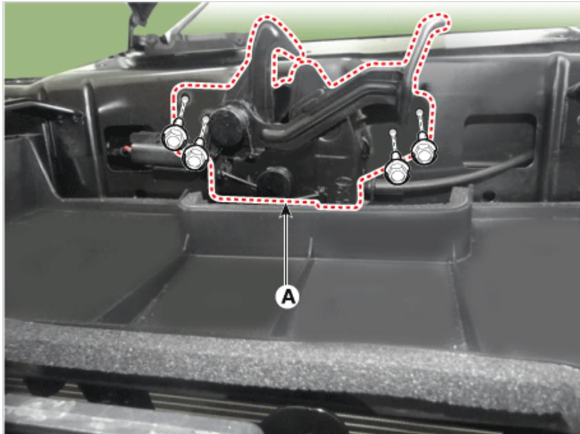
3. Disconnect the hood latch cable (A).
