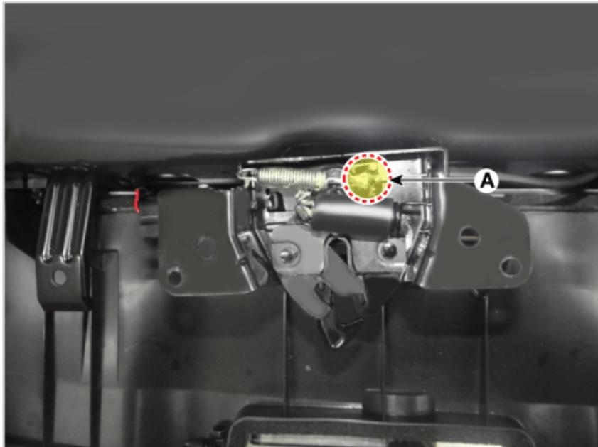
4. Disconnect the hood latch connector (A) after loosening the mounting screw.
